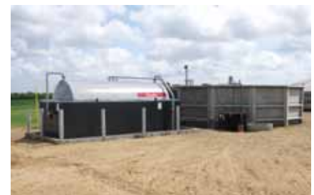
Acid tank and processing tank of the slurry acidification system from J.H. Staldservice A/S.
